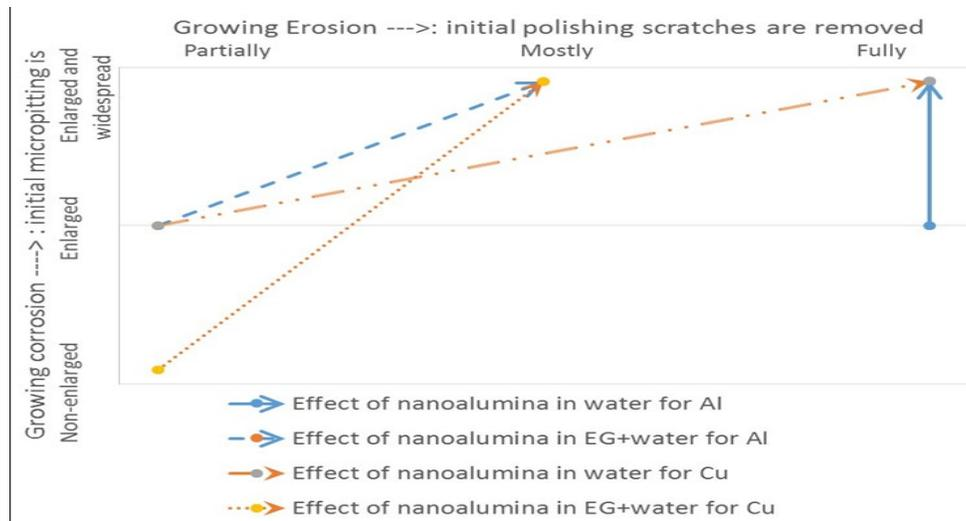
Figure 5. Evolution of erosion and corrosion effects (as assessed, respectively, by microscopy-image removal of initial polishing-scratches and enhancement of initial micro-pitting) from 2%-nanoalumina addition in each coolant fluid (water and 50% ethylene glycol in water) jet-impinged on aluminum 3003-T3 and copper alloy110.
