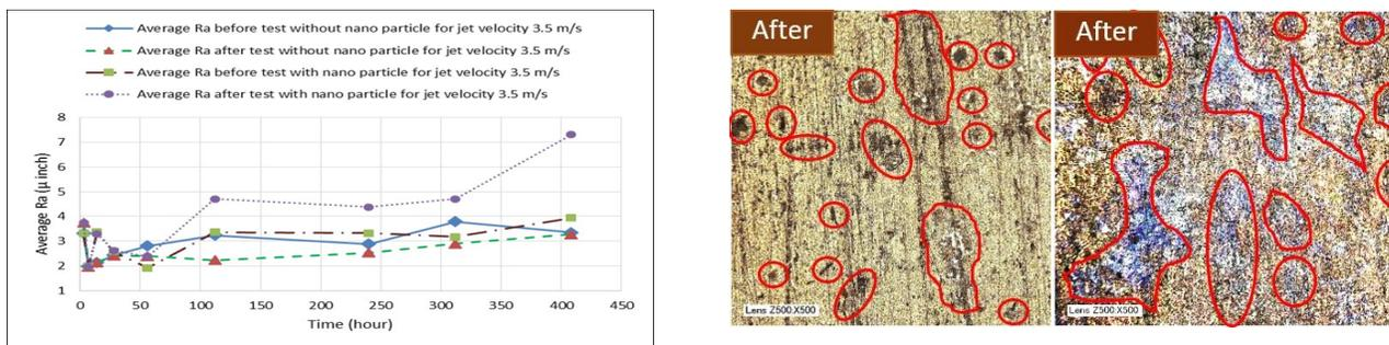
Figure 4: Average Ra for copper 110 after 3, 7, 14, 28, 56, 112 and 408 hour-treatments with distilled water, and its nanofluid of 2% nano-alumina, and optical microscopy images (Magnif.:500X) before and after test of 408 hour-test (left image: after test with nanofluid; right image: distilled water only). Flow speed 3.5 m/s.
