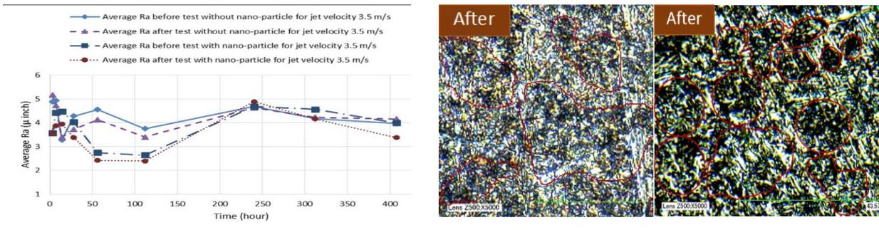
Figure 3. Jet-impingement tests: Ra roughness for 3003-T3 aluminum before and after 3, 7, 14, 28, 56, 112, 240, 312 and 408 hours with 50/50% Ethylene Glycol in water (EG/w), and with its nanofluid of 2% nano-alumina and optical microscopy images (Magnif:5000X) for 408 hour-test (left image: after test with EE/w nanofluid; right image: EG/w). Jet-speed speed 3.5m/s.
