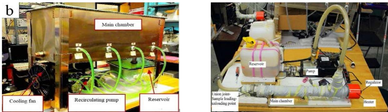
Figure 1. Jet-impingement (left image) and through-flow test-rig (right image) for testing of nanofluids effects [3-4]
